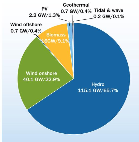
FIG 12: TECHNOLOGY SHARE OF EU INSTALLED RENEWABLE POWER CAPACITY IN 2020 (GW) - TOTAL 487.2 GW
